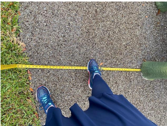
Image 4. Distance between play sculpture and safety surfacing edge is approximately 2.5ft and must be corrected to meet a minimum of 6ft of safety surfacing around the entire play sculpture.
