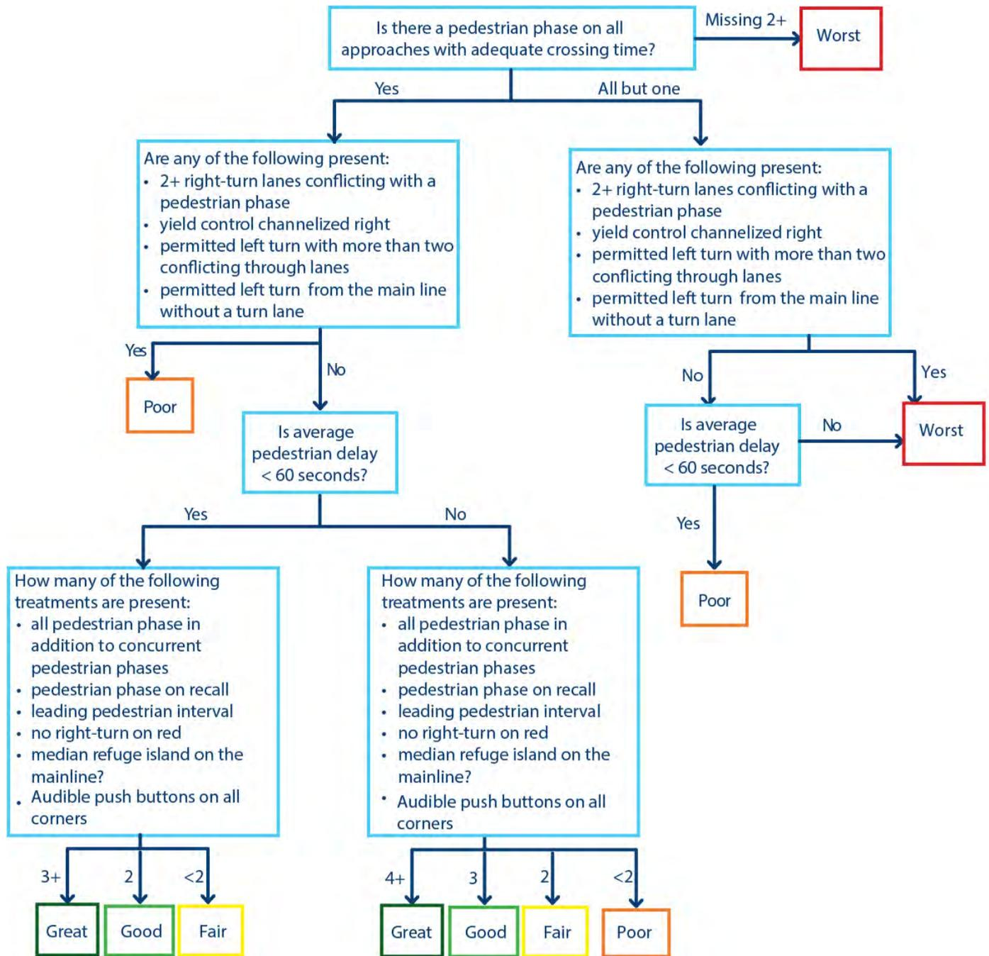
**FIGURE 9 PEDESTRIAN SIGNALIZED INTERSECTION ACCOMMODATION - EIGHT OR MORE LANES ON THE MAINLINE**
